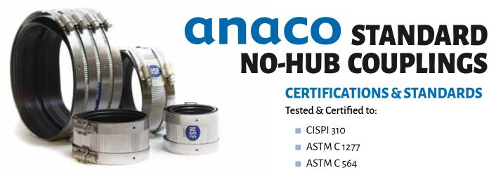
Anaco No-Hub couplings consist of a 300 Series stainless steel shield, clamp assembly and a Neoprene gasket. Coupling sizes range from 1½" through 15" diameters.
