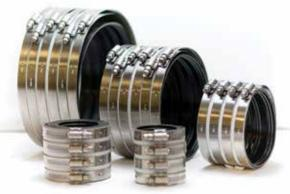
Husky HD 2000 Couplings have a slightly thinner shield than the Husky SD 4000. They consist of a 304 stainless steel shield, clamp assembly and a neoprene gasket. The 305 stainless steel 5/16" screw requires 80-inch pounds of torque. Sizes: 1½"-10"
